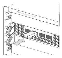
Figure 22: Installing a CFP2 Module (CFP2 LR4 module shown)
